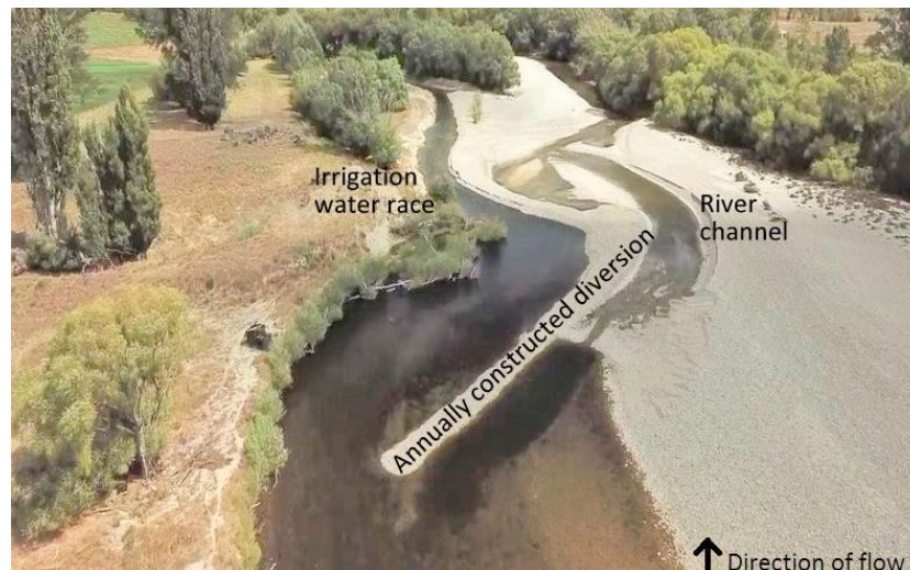
Figure 2.3. Aerial view of the water abstraction point 3.M, temporary Galloway diversion during water abstraction and seasonal low discharge period, 2019 occasion - DA. The direction of flow is away from the reader. Most water flows into the irrigation water race and <50% of the discharge flows into the main river channel.
