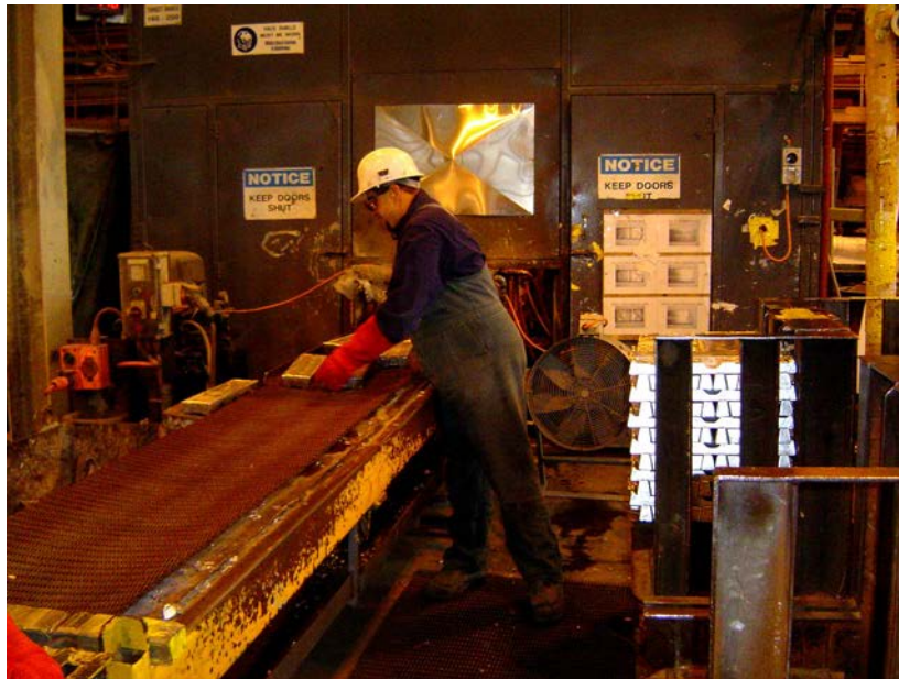
Figure 11 – Casting worker manually stacking zinc slabs
