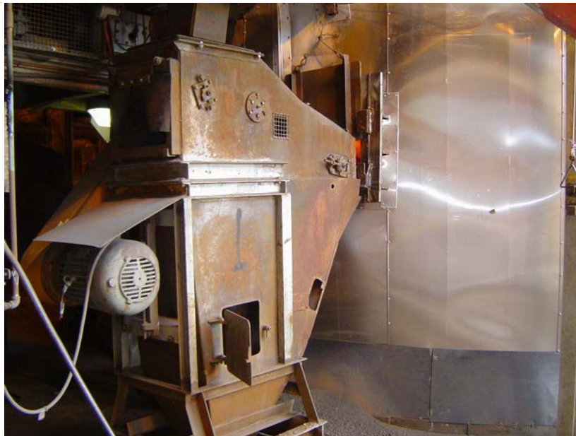
Figure 8 – Slinger Feeder feeding the Roaster
